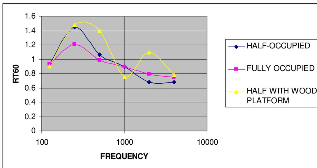
Notice that in all three cases, the reverberation time is close to the target value of 1.1 to 1.2 seconds at 2 kHz, which is the most important band for speech intelligibility. The increase in reverberation time at low frequencies is no more than 66% in any case. This sanctuary will have a pleasant sound for your worship style. The use of a more absorptive ceiling material is not recommended, as it would make the room too acoustically dead.
