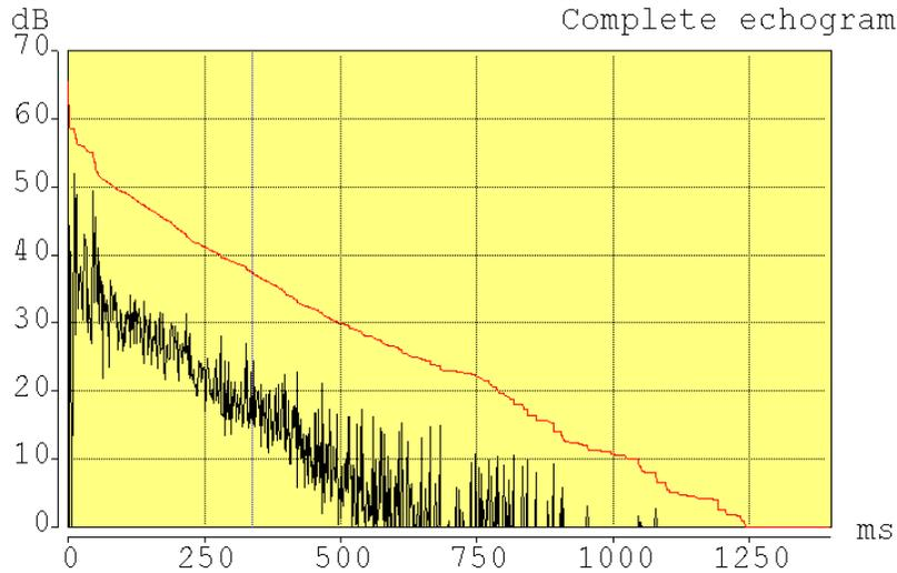
The continuous curve represents the reverberant sound level as it decays. Any humps in that curve might represent echoes, if they occurred after 65 milliseconds and were sufficiently loud compared to the original sound. Notice that there is over 38 dB between the original sound and the first bumps in the curve after 65 milliseconds, indicating that echoes will not be a problem for any program material.
